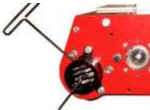
Hydraulic Motor Side B Eccentric set at setting 3
