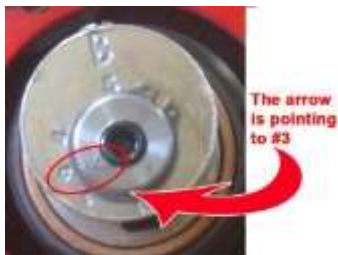
Hydraulic Motor Side B Eccentric set at setting 3
