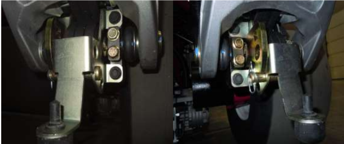
These two views show the TORO Triflex Counterbalance adjustment.
